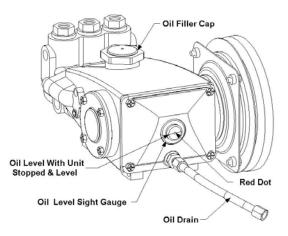
2. After **50 hours** operation, change the crankcase oil with CAT Pump Crankcase Oil, (Part # 13-000). Change the crankcase oil every **500 hours** thereafter.
